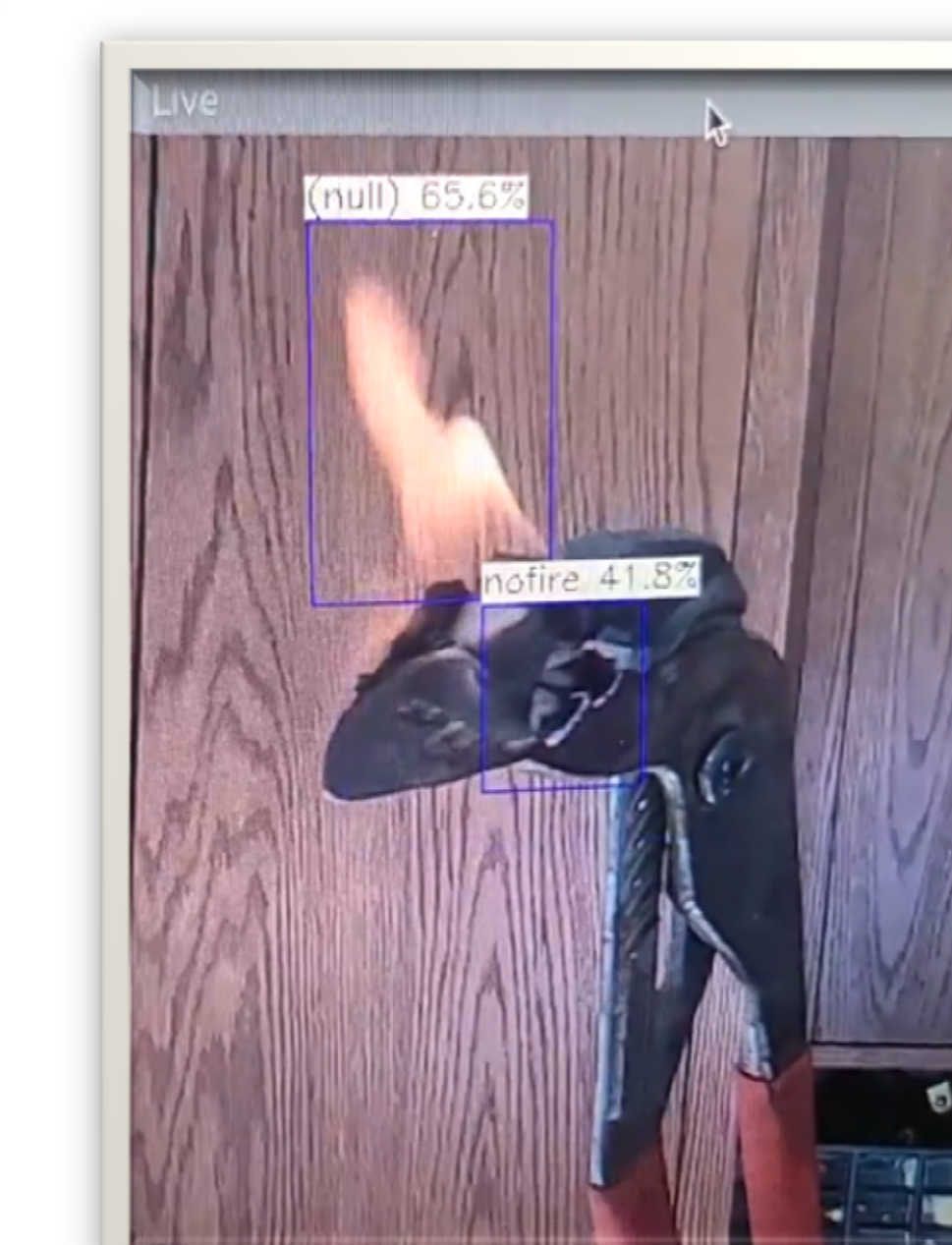
Raspicam Mounted with implemented fire detection and camera servo
